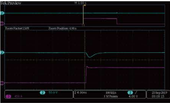
CH2: Output voltage waveform; CH3: Output current waveform EVWB-500-1000 (500kW, 1000V, 1000A) transient test: It can be seen from the waveforms that under a 500V output state, when a 900A current load is suddenly applied, the voltage recovery time is approximately 3ms.
