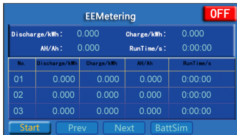
Fig. 3-9-3 Electric energy metering interface
